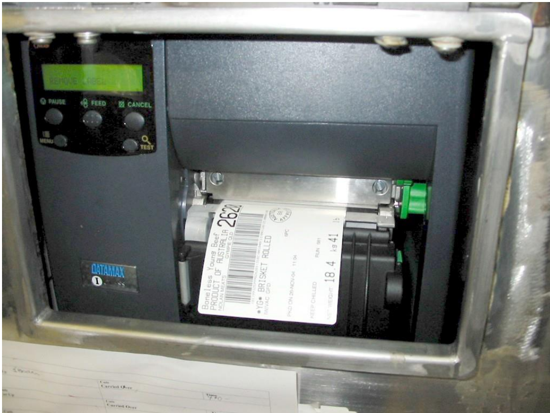
Figure 13 – Datamax Printer Operating in Cabinet
